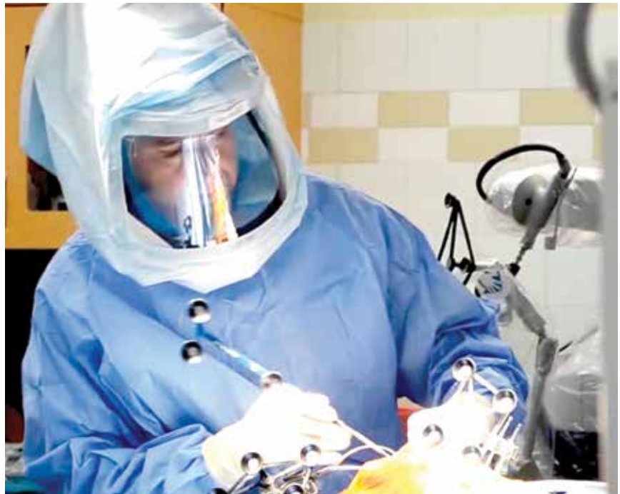
The surgeon's hands, the surgical instruments and the surgical site are marked with sensors which update the robot about movements of the surgeon's hands.
